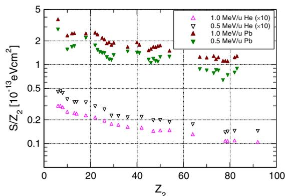
Fig. 1. Stopping cross section per target electron for 1.0 and 0.5 MeV/u Pb [15] and He [8] ions versus atomic number of the target material, from [3].
