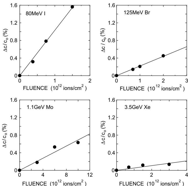
Fig. 2. Fluence dependence of normalized lattice expansion,  $\Delta c/c_0$ , for the irradiations having same  $S_e$  and different ion-velocity. The solid lines are to demonstrate the  $c$ -axis lattice parameter increases linearly with increasing ion-fluence.
