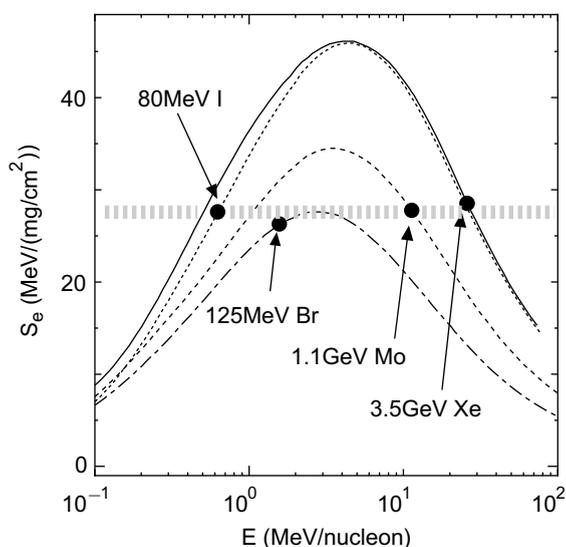
Fig. 1. Electronic stopping power,  $S_e$ , plotted as a function of energy. The electronic stopping power is estimated using SRIM2003 [13,14]. The  $S_e$  values for the present irradiations are indicated by full circles. The gray dotted line is to demonstrate that values of  $S_e$  for the present irradiations are almost the same.
