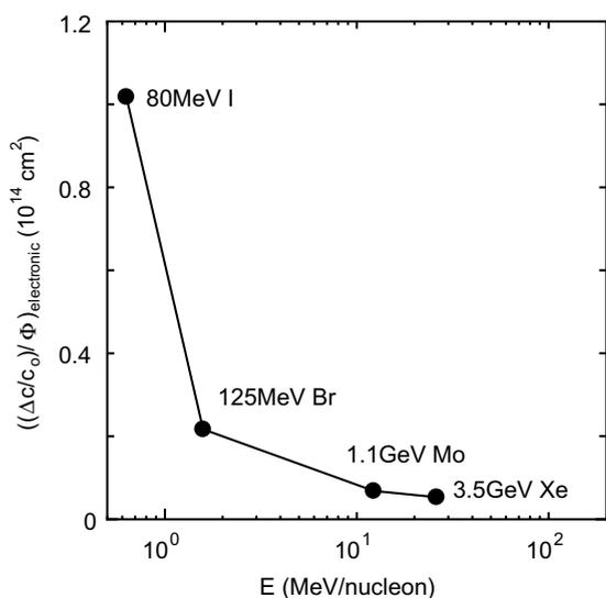
Fig. 3. Contribution of electronic excitation to lattice expansion per unit fluence,  $((\Delta c/c_0)/\Phi)_{\text{electronic}}$ , plotted against energy per nucleon.
