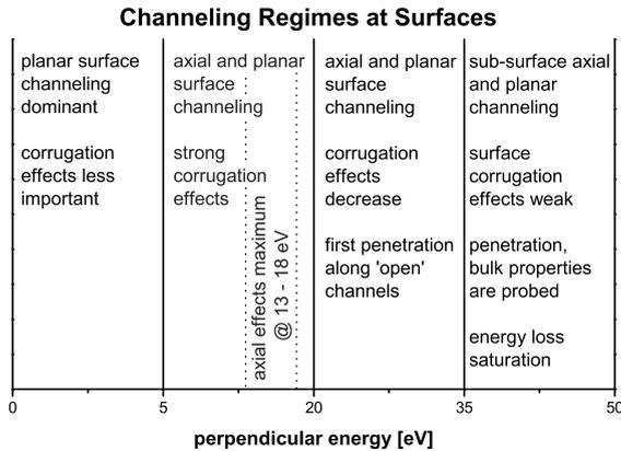
Fig. 5. Road-map of surface channeling regimes depending on the perpendicular energy obtained from the two scattering systems under consideration.
