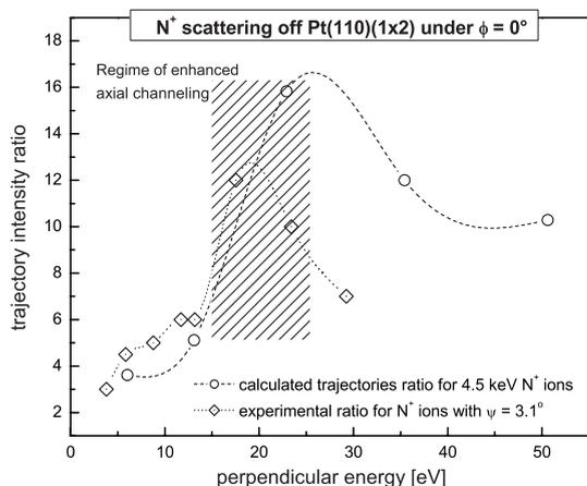
Fig. 3. Intensity ratio of particles scattered *on-top* and *in-row* the surface channels. The ratio indicates the strength of *axial channeling*. Experimental and calculated intensities are compared when varying the perpendicular energy of the primary ions. Lines are drawn to guide the eye.
