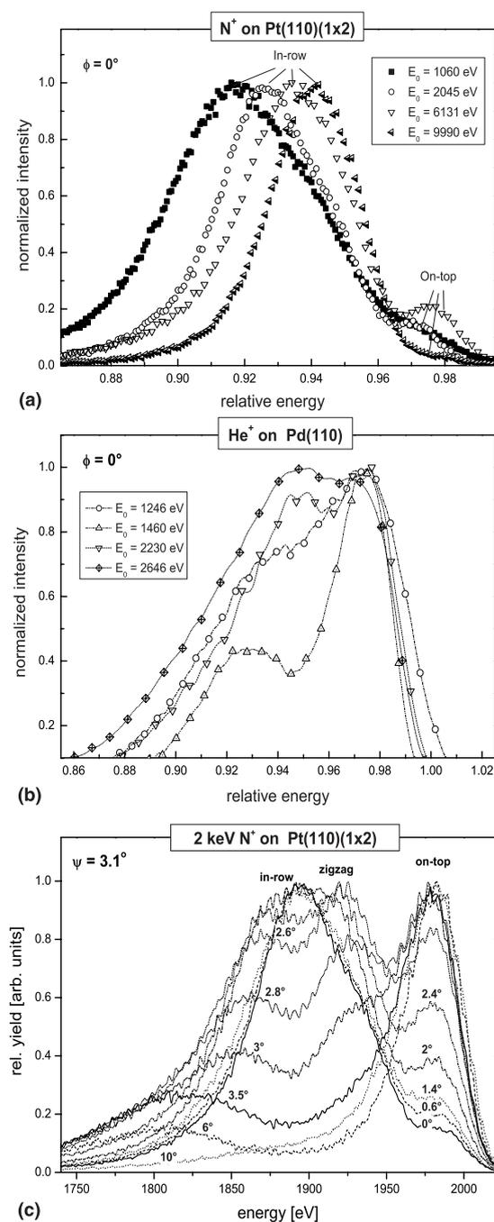
Fig. 1. Experimental energy loss spectra along the  $[1\bar{1}0]$  surface channel for different primary ion energies: (a)  $N^+$  on Pt(110)(1 × 2), (b)  $He^+$  on Pd(110). Part (c) shows a sequence of nitrogen ions scattering of Pt(110) with constant primary energy, varying in small steps the azimuthal angle close the  $[1\bar{1}0]$  surface channel.
