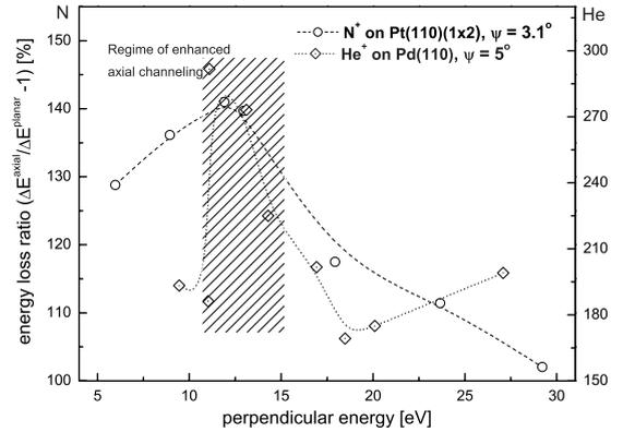
Fig. 2. Experimentally obtained energy loss ratio comparing the energy loss under axial and planar channeling conditions when varying the perpendicular energy. Lines are drawn to guide the eye. The angle of incidence is kept constant. Similar behavior is found for MeV nitrogen ions [16].
