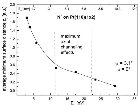
Fig. 4. Average minimum surface distance depending on the perpendicular energy for nitrogen atoms scattering along the  $[1\bar{1}0]$ -surface channel of Pt(110). Values are obtained from Monte Carlo trajectory calculations [5,9].
