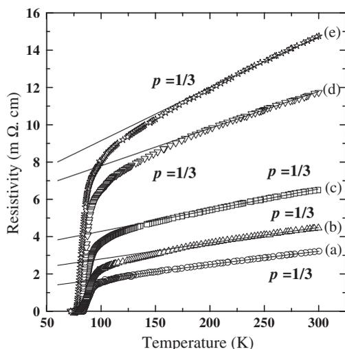
Fig. 5. VRH fit with the experimental temperature dependence of normal state resistivity for sample Q2 with fluence (a) zero, (b)  $7 \times 10^{13}$  ions/cm<sup>2</sup>, (c)  $2 \times 10^{14}$  ions/cm<sup>2</sup>, (d)  $7 \times 10^{14}$  ions/cm<sup>2</sup> and (e)  $1 \times 10^{15}$  ions/cm<sup>2</sup>.
