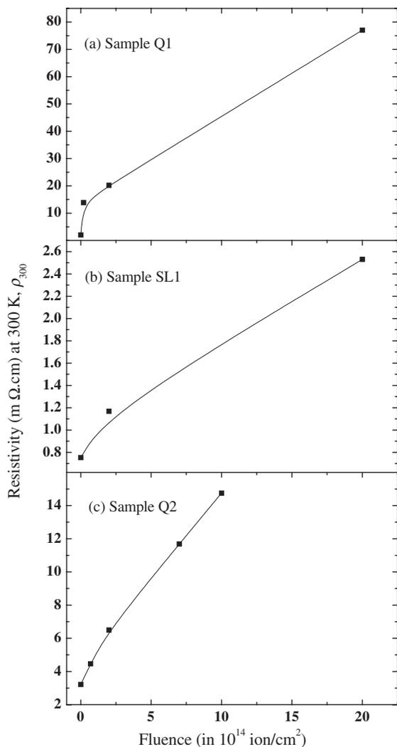
Fig. 1. Variations of room temperature resistivity ( $\rho_{300}$ ) with irradiation fluence for (a) sample Q1, (b) sample SL1 and (c) for sample Q2.
