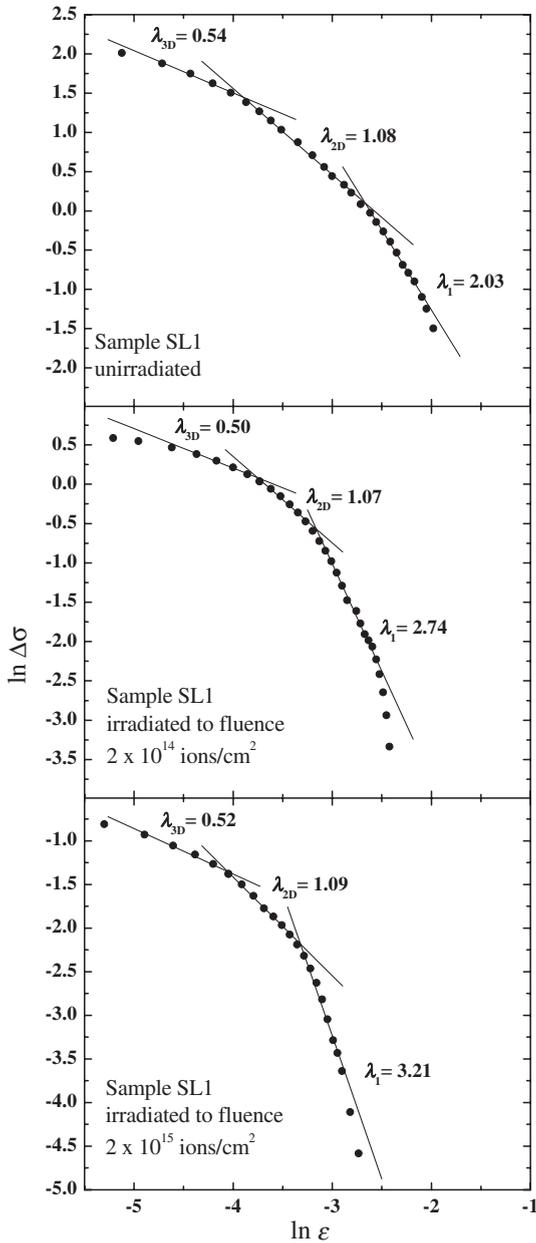
Fig. 3. Irradiation induced modification of different regions of paraconductivity for the sample SL1.
