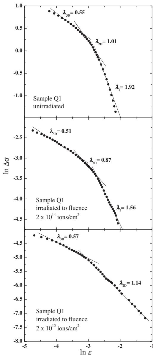
Fig. 2. Irradiation induced modification of different regions of paraconductivity for the sample Q1.
