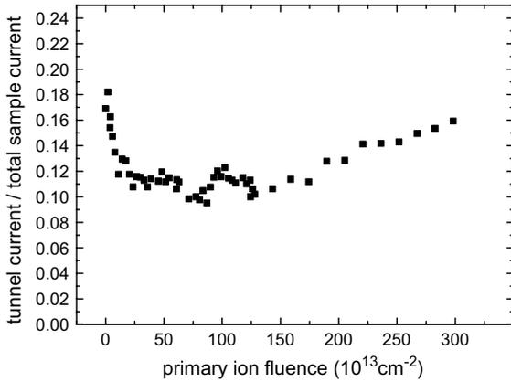
Fig. 2. Measured tunneling current as a function of accumulated total primary ion fluence. The decrease at the beginning is due to removal of surface contamination, after a constant region the signal increases because of degrading silver thickness.
