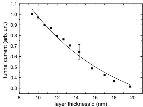
Fig. 3. Measured tunneling current as a function of the silver top electrode thickness as calculated from the primary ion fluence and literature data of the sputter yield.
