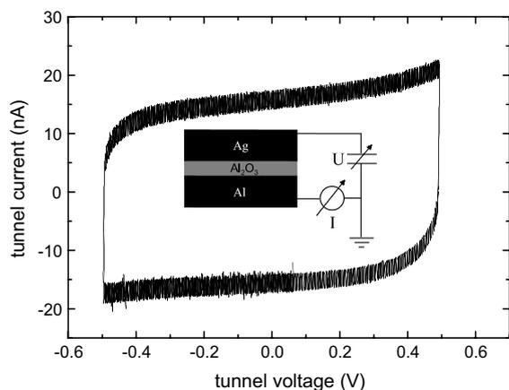
Fig. 1. Dynamic  $I$ - $V$  curve characterizing the electrical properties of the MIM-junction measured at a scan rate of 200 mV/s.
