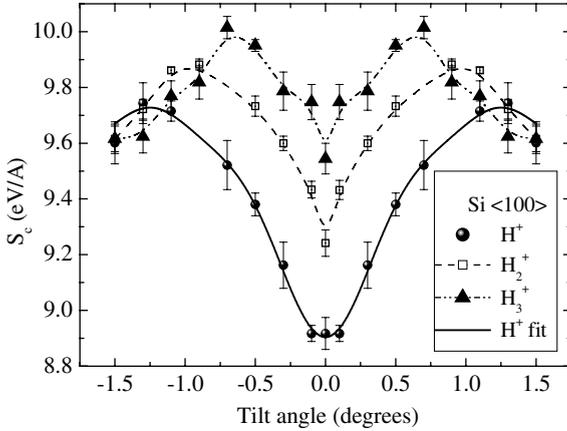
Fig. 2. Channeling stopping power as a function of the tilt angle. Full circles correspond to  $H^+$  ions, open squares correspond to  $H_2^+$  molecule and full triangles to  $H_3^+$  molecules. The full line is the fitting to the  $H^+$  data (using two gaussian functions) and the other lines are plotted only to guide the eyes.
