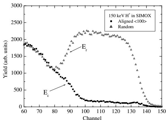
Fig. 1. RBS/channeling spectra of the SIMOX target. Open triangles stand for random spectrum and the squares stand for the  $\langle 100 \rangle$  channeling spectrum.
